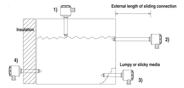
The drawing shows how the sliding connection can be used for at least 4 applications:
